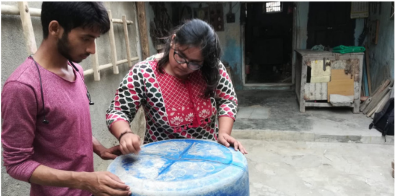
marking of holes on the drum
