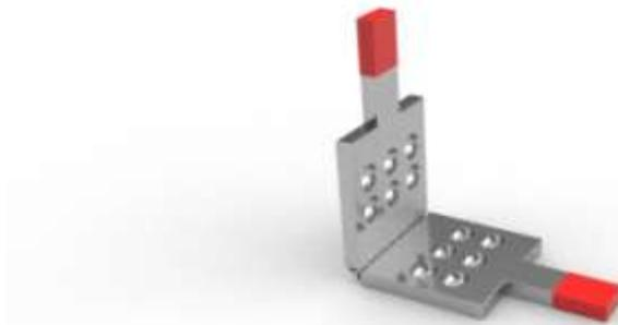
In this device the content was quiet same as 2<sup>nd</sup> research but it had a 6 holes in single surface and there are having 6 nuts can crack in single operation, but the problem is having that load can be distribution can be happen. The 1<sup>st</sup> third hole can be crack easily, but 2<sup>nd</sup> three holes cannot have proper presser so they cannot crack properly.
