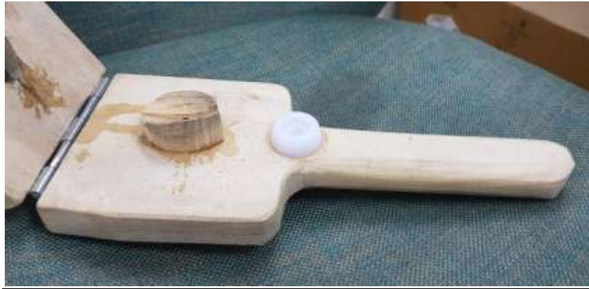
In this device we had research and also this device is our current device and also we can use in our experiment. This device we had use small blade and this blade is break the nuts in two parts. In this operation we had hold the nut on blade and press with bottom surface and on opposite side the embossing part can help to press breaks the nuts. But there is a problem that the nuts cannot crack properly but our team can solve the problem as soon as possible.
